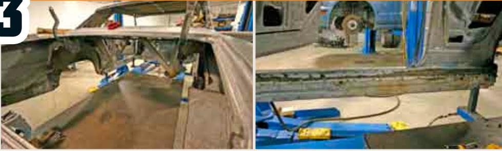
Shown here is our new Flintstone mobile (minus the stone wheels). Once the floor is cut around the edges, it's necessary to employ a drill bit—or better yet, a spot-weld cutter—to properly and carefully remove the remainder of the floor pan that's welded to the rocker section.
