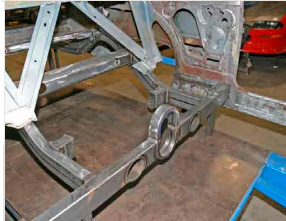
Once the axle centerline was determined, the rear frame was mocked up under the Nova, measured for length, and trued to the vehicle itself. After the crossmember and the rear portion of the frame were cut, it was tack welded into place (the frame will be fully welded once
